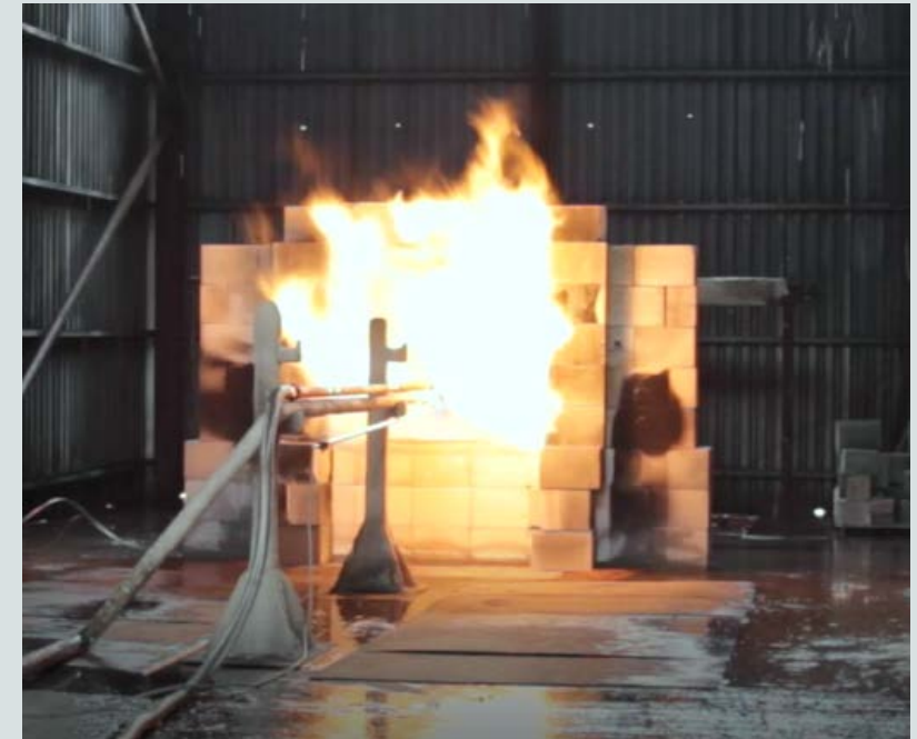
Jet fire test done on 2-part paint system, being performed to ISO 22899-1 test standards.
